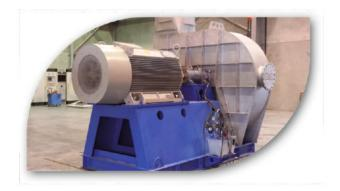
In mechanical vapor compression the generated vapor (saturated steam) from the evaporator will be boost by using a MVR-Fan to a higher pressure level and fed back as heating steam to the evaporator again. Thus the fan operates as a heat pump.
