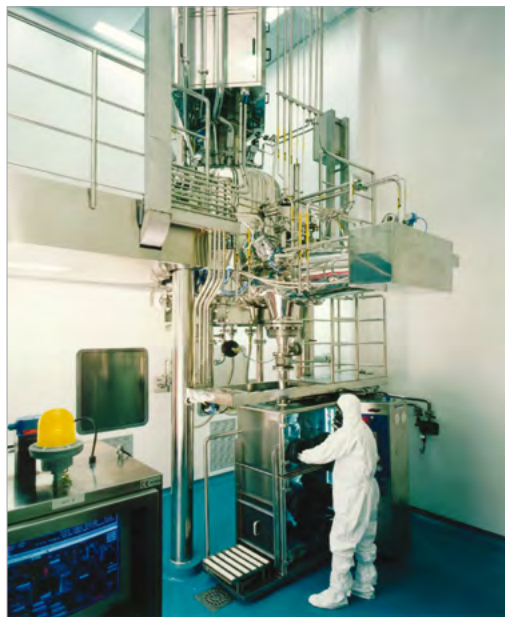
FILTRODRY FEP/XD 150 1.5 SQM NUTSCHE FILTER DRYER IN STERILE VERSION
