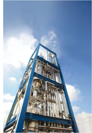
DOUBLE STAGE SKID-MOUNTED THIN FILM EVAPORATOR FOR AGROCHEMICAL CONCENTRATION
