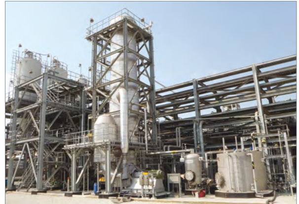
SINGLE EFFECT MVR FALLING FILM EVAPORATOR FOR WASTEWATER CONCENTRATION
