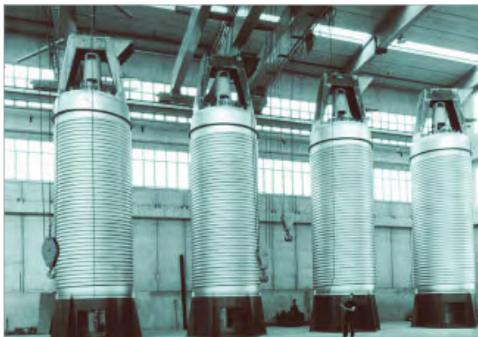
120 M 3 BIO REACTOR STUDIED AND DESIGNED WITH OUR BIOCHEMICAL ENGINEERS
