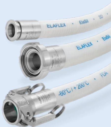
Silicone hose for high media purity requirements with smooth lining of platinum-cured, translucent, phthalate-free silicone. Highly flexible, kink and vacuum resistant, large temperature range -60°C up to +200°C (depending on medium). Conform to FDA, USP Class VI and 3-A Sanitary Standard, suitable e.g. for cosmetics, pharmaceuticals and foodstuffs. Steaming out for cleaning and sterilisation possible, autoclavable.
