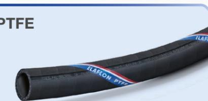
The star among our EN 12115 'Ω/T' hoses: Electrically conductive, seamless lining of Teflon® PTFE, for all commonly used media up to +150°C (depending on medium). Conforms to FDA and USP Class VI.
