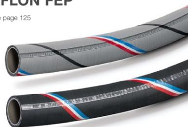
Universal hose with seamless, transparent lining of Teflon® FEP. Suitable for all common media up to +100°C, briefly up to +130°C. Conforms to FDA and USP Class VI.
