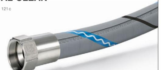
Universal hose 'CLEAN' with electrically conductive, seamless UPE lining and light grey cover. Suitable for a large range of media, up to +100°C. Corresponds to EN 12115. Conform to FDA. Steaming out for cleaning and sterilisation up to +130°C, max. 30 min. (open system).
