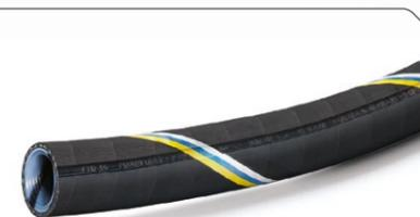
Universal hose with seamlessly extruded, helically wound lining of Teflon® PTFE virginal, white. Suitable for all common media in use. Exceptional flexibility and tight bending radii. With patented inner conductive OHM spiral stripe for clean media and highest electrostatic safety.
