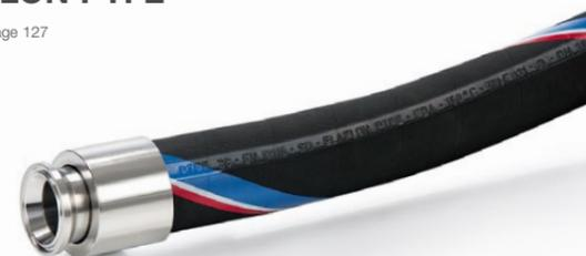
Universal hose with electrically conductive, seamless lining of Teflon® PTFE, for all commonly used media up to +150°C (depending on medium). Corresponds to EN 12115. Conform to FDA and USP Class VI. Steaming out for cleaning and sterilisation up to +150°C, max. 30 min. (open system).
