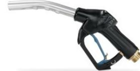
Corrosion resistant nozzles with automatic shut-off. Flowrate up to 60 l/min. Inner parts of stainless steel, seals of Teflon®
