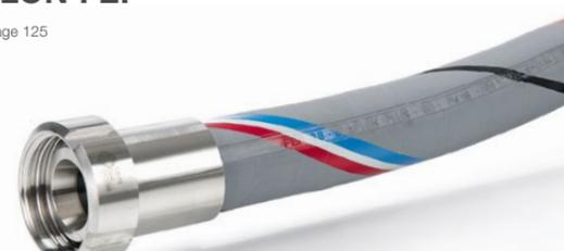
Universal hose with seamless, transparent lining of Teflon® FEP, for all commonly used media Medien up to +130°C (depending on medium). Corresponds to EN 12115. Conform to FDA and USP Class VI. Steaming out for cleaning and sterilisation up to +150°C, max. 30 min. (open system).
